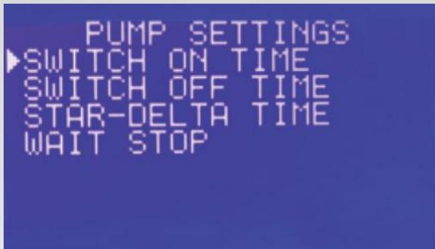
**c.  $\lambda / \Delta$  Time:** On Star-Delta Ramp-Up type motors, star-delta transition time is configured on this parameter. Default factory setting is 5 seconds.
